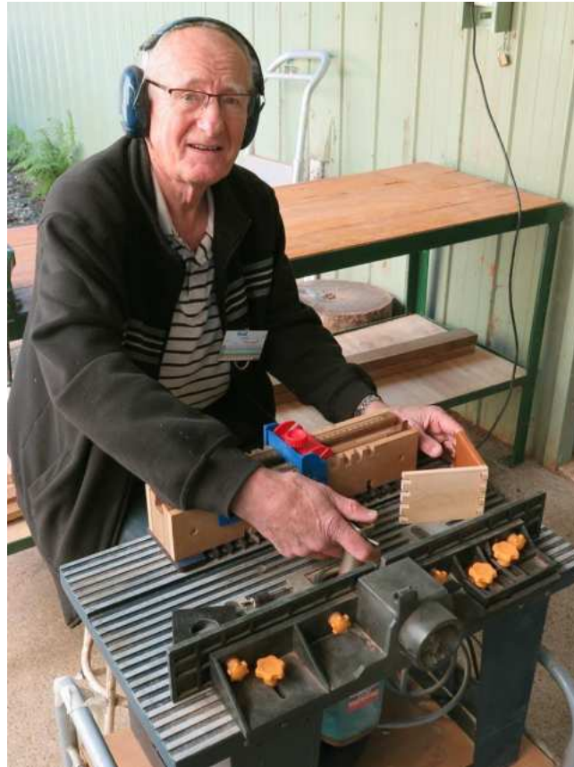
Rod G using a dovetail template device to cut dovetails for a box
