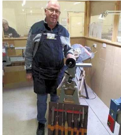
Dick is making a magnetic lathe tool rack to hold gouges and tools for each wood lathes
